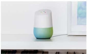
Similar in shape to an oversized salt shaker, the Home performs more or less the same functions as the Echo. It uses a set of far-field microphones to continuously listen to users and answer questions, control music, control some connected devices and even stream media from a smartphone or tablet to a Google Cast.
