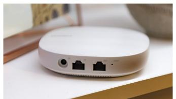
The Connect Home uses Eero-style mesh networking, meaning a single router provides up to 140 square metres of coverage while a combination of three routers covers 418 square metres. In addition, the SmartThings platform allows it to communicate with other devices via Bluetooth 4.1, ZigBee or Z-Wave as well as wifi, providing the control Samsung appliances, Philips Hue lighting and Netgear Arlo cameras, among others.
