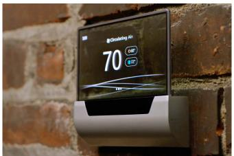
The GLAS offers a translucent touchscreen as well as voice control, and packs sensors allowing it to detect whether people are in the room or not, and if not to turn the HVAC system on or off. It can also check air quality and energy usage. Of course, Cortana allows users to simply speak to the GLAS, and one can also control it by speaking to their phone.
