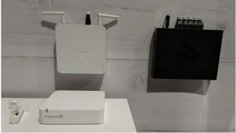
The CA-1 features ethernet, wifi, ZigBee and serial connectivity, and leverages on the Control4 database of thousands of 3rd party devices. An optional Z-Wave module adds compatibility with Z-Wave-enabled devices such as door, window, water, flood and temperature sensors, as well as electrical outlets and dimmer outlet modules. Power over Ethernet (PoE) allows installation anywhere with a single network cable.
