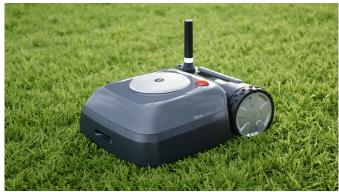
According to the company, the Terra uses Imprint mapping technology in mow the lawn just like people do, navigating a yard in straight, back-and-forth lines. The robot even remembers where it is in the yard and where it still needs to cover, in case it runs out of battery. In case of such a situation, the robot returns to base to recharge before resuming on mowing duties.
