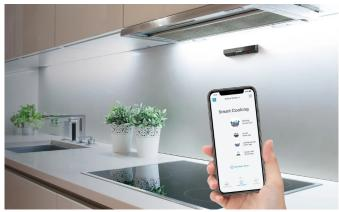
At first glance the Sense appears to be a fairly simple device. It features a slim, one-button design, and can be easily mounted above a cooktop, wall or under the cooker hood. However Safera says it carries a "powerful" processor able to analyse data from over 20 sensors allowing it to work out stove temperature, air quality, cooker power consumption and even human activity around the stove, and is compatible with both electric and gas stoves.
