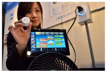
The Wall Street Journal reports the company has a prototype "smart socket" using RFID and authentication technologies to track energy use by appliance, limit consumption by time, user or device and even block energy access to non-authorised plugs.
