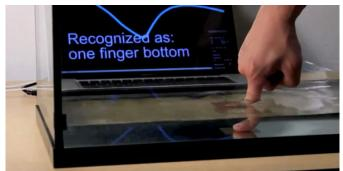
Touché uses Swept Frequency Capacitative Sensing (SFCS), a technology derived from modern smartphone touchscreens. It recognises a wide range of different gestures, with each gesture (tapping, pinching, grasping) having different "capacitative profile" to trigger different functions.
