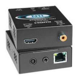
NTI's **HDMI HDBase-T extender** transmits an uncompressed high speed digital HDMI signal, IR, and optional SPDIF digital audio up to 328 feet (100 meters) over a single CAT5e/6/7 cable.
