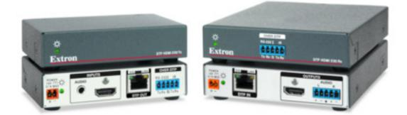
Extron Electronics announces immediate availability of the **DTP HDMI 230** twisted pair extender for transmission of HDMI, audio, and bidirectional RS-232 and IR control signals up to 230 feet (70 meters) over a single CAT 5-type cable.
