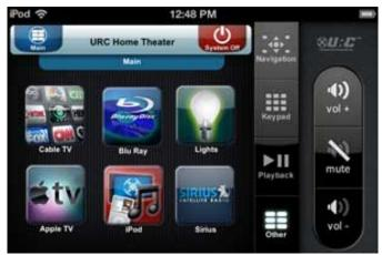
The app uses local area IP networks and transforms iDevices into AV, home theatre and lighting controllers. The GUI is customisable, allowing installers to design control screens as per customer requirements and preferences.
