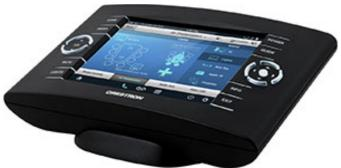
The touchscreen features illuminated pushbuttons for programming macros such as volume adjustment, channel selection and on-screen menu navigation options. Rava SIP intercom technology also allows it to handle hands-free full-duplex VoIP communications between any two Rava-enabled Crestron touchscreens and 3rd party door stations.
