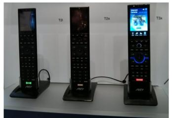
The T3x remote control combines a 3.5-inch touchscreen with programmable hard buttons, and is designed for simple integration with any installation. It features a dual RF platform with one-way control via 433MHz RF or bi-directional communication via 2.4GHz ZigBee. Wifi support allows web browsing and wireless program updates, while furthe features include integrated grip sensors, accelerometer and haptic feedback within the touchscreen.
