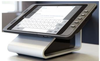
The device replaces the top half of the 2-part iPad mini sleeves for iPort's LaunchPort inductive charging system. Once connected to the sleeve it uses Clear Connect wireless technology to communicate with any Lutron RadioRa 2, HomeWorks QS or Caseta bridge or router.
