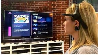
Based on a cheap brainwave-reading headset, the headset has users turn on and operate the app through either concentrating or relaxing their minds.
