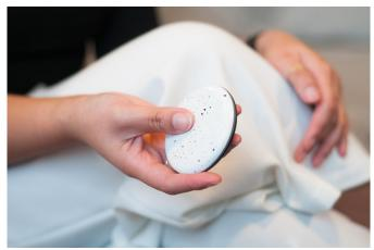
The actual Flipp remote is a palm-size disc. It does exactly four things, namely pause/play music, control volume, skip songs and skip playlists. It has no buttons, meaning control is tied to specific motions based on how one is holding the Flipp.
