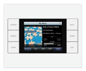
It is touch-screen based and controls any device on an IP home network, from personal servers to energy monitoring devices and media players-- via preprogrammed modules. Network connection is via eithernet or wifi.
