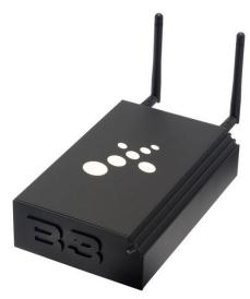
It carries a 1.2GHz ARM processor together with 512MB of RAM, while Excito says power consumption is as low as 5W. The device can handle up to 4TB of file sharing and storage.
