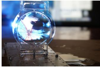
A "colloidal display" consists of the surface of a soapy bubble (or "membrane screen"), over which a projector beams images. In this case the bubble is made out a complex colloid solution, and is far stronger than anything from your bubble bath or dish washer.
