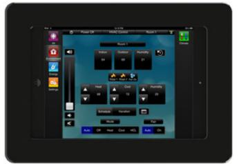
The wifi-connected docks consist of a mounting plate and back-box with low-profile, magnitically attached bezels. The dock powers the iOS device, whose touchscreen allows for wireless navigation and control of Savant automation and control systems.
