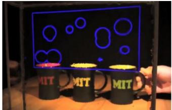
The new system embeds nanoparticles in the transparent material. These tiny particles can be tuned to scatter only certain wavelengths, or colors, or light, while letting all the rest pass right through. The glass remains transparent enough to see colors and shapes clearly through it, while a single-color display is clearly visible on the glass.
