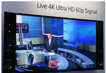
Live events in New York City were captured with the Sony F55 4K camera, and HEVC encoded using Cisco's Videoscape AnyRes -- with enhanced support for 4K and HEVC. The live stream was transported from New York to Las Vegas through a fiber optic network. The stream was then be delivered to the Las Vegas Convention Center, decoded with a Cisco set-top box with 4K support, and displayed on Sony XBR 4K Ultra HD TVs.
