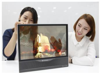
The flexible OLED panel features 1200 x 810 resolution with a 30R curvature radius. Made using a "high molecular substance-based polyimide film" backplane to achieve both flexibility and thinness, one can roll the display to a radius of 3cm without affecting its functionality.
