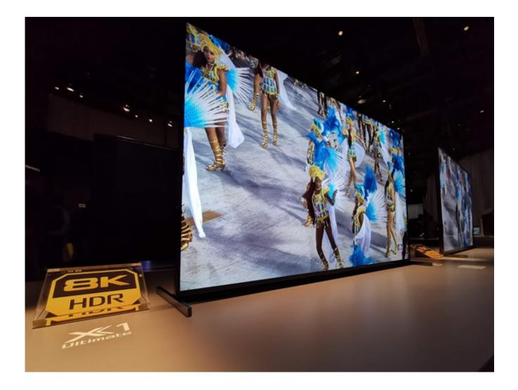
Essentially, the frame tweeter vibrates the frame of the TV to emit sound, giving viewers the feeling sound is coming directly from the screen. Available in 85- ad 75-inch models, the ZH8 also features the X1 Ultimate picture processor and 8K X-Reality PRO technology to upscale content to what Sony claims is "closer to 8K quality," while ambient optimisation automatically adjust image brightness according to the ambient lighting of the room.
