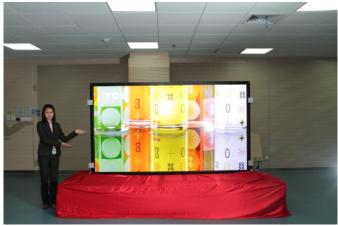
The giant display carries 4K by 2K (4096 x 2160 pixels) panels, active 3D technology and dynamic backlighting. It also has multi-touch functionality, and produces 800 nits of brightness while reproducing 92% of NTSC colour gamut.
