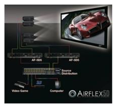
The AirFlex5D system aligns images from multiple projectors vertically and horizontally. It handles image resolutions of up to 1920x1200 with dual-channel geometric image correction, de-interlacing, scaling and image enhancement.
