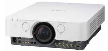
The technology uses a blue laser light source to excite a phosphorous material into generating white light. The 3LCD optical system splits the white light into RGB, producing 4000 lumens of light at WUXGA (1920x1200) resolution and what Sony claims is "bright and vivid color reproduction."
