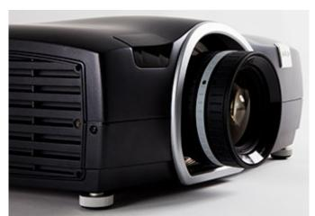
According to the company it carries a lamp-based single-chip DLP, a co-development with Texas Instruments, allowing the projection of 2560x1080 images without need for additional anamorphic lenses. The format uses 78% more pixels for native 2.37:1 compared to standard 1080p projectors with a Blu-ray 2.37:1 format movie.
