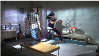
Currently in proof-of-concept prototype stage, RoomAlive uses a commodity wide field of view projector, a Kinect sensor and a PC to build a projector depth-camera unit (aka procam). The Kinect and PC capture and analyse a 3D model of the room required for the projection of images users can interact with, and keep track of all users-- in other words interactive projection mapping.
