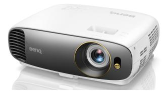
The projector uses 0.47-inch single-DMD-chip DLP technology together with BenQ CinematicColor technology and an RGBRGB colour wheel to hit 96% coverage of Rec. 709 colour gamut. In total it can push 8.3 million distinctive pixels, with 2200 ANSI lumens brightness and 1000:1 contrast ratio.
