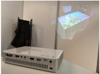
The M550 Plus beams 1280x800 resolution images in dimensions of to 200-inch diagonal from 0.5 - 3m distance. It offers 3D as well as regular 2D images, and promises a battery life of up to 3 hours on a single charge. The contrast ratio is 1000:1, while lamp life clocks at around 20000 hours. Audio is also included via 3W speakers.
