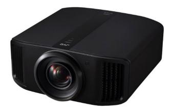
The DLA-NX9 combines 8K e-shift pixel shifting with a 100mm diameter 18-element, 16-group all-glass lens to ensure high resolution into the extreme corner of the screen. Five low dispersion lenses suppress chromatic aberration and bleeding, while a variety of techniques reduce light scattering and light diffraction, improving brightness and black levels.
