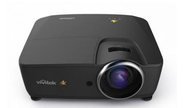
The projector features a Texas Instruments 0.66-inch 4K DLP DMD chip able to generate 8.3 million individual pixels. Also included are DLP DarkChip3 and BrilliantColor refinements for deep black levels and vibrant cinematic images. To resolve a 4K 1-pixel line pattern, the HK2288 uses eXpanded Pixel Resolution (XPR) technology employing 4.15 million (2716 x 1528) mirrors capable of switching over 9000 times per second to deliver two discrete pixels for each mirror per frame.
