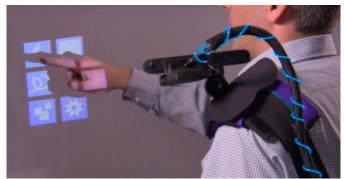
The projector sits on the user's shoulder, beaming images via pico projector on walls the wearer can interact with as a fully interactive surface. Handling interactions is a depth-sensing camera.
