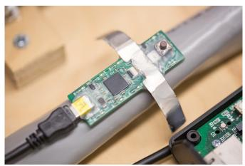
The system consists of 5 small sensors placed above or near power lines coming into the house. The sensors pinpoint each light or appliance based on power use, before pushing the data to a companion app in realtime. Each sensor is self-calibrating, and can pinpoint the strongest electrical signals. In turn the system can distinguish between each type of light, appliance or device based on unique signals.
