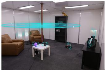
Dubbed "Quasistatic Cavity Resonance for Ubiquitous Wireless Power Transfer," the technology is free roaming, meaning one can move around the room and their smartphone will immediately start charging, with no need to be close to a wireless charging pad. It is also very efficient (around 40-95%, depending on the receiver's position in the room) and can deliver 1900W of power before the specific absorption rate (SAR) becomes dangerous for human beings.
