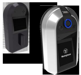
While looking like any other smart door lock, the Nucli packs an integrated outdoor camera, motion detection, fingerprint reader, inner and outer touchscreens, accelerometer, VoIP communications and doorbell. Wireless connectivity comes through Z-Wave, Bluetooth and wifi, and Westinghouse says it can be used to control Z-Wave devices (via custom touchscreen swipes) either individually or in groups.
