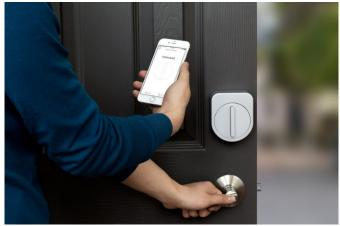
Once attached to the lock, the Sesame pairs with smartphones via Bluetooth LE and companion app. An additional Wifi Access Point accessory adds internet connectivity for remote locking and unlocking, while included lithium batteries promise up to 500 days of use.
