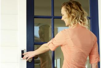
Like the original Video Doorbell, the Pro connects to home networks via wifi to provide homeowners with smartphone alerts in case someone is at the door. It also allows users to answer the door via phone with a video call, reducing the need to actually get up for checking duties (should one actually want to do that, of course).
