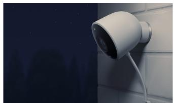
As the name might suggest, the Nest Cam Outdoor features a weatherproof casing and more mounting options, including magnetic and screw-on mounts for attachment outside a building. However one has to keep in mind the camera requires constant power via plugging to an outlet.
