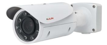
Available in 2 versions (the ZR8022X20 with 20x 4.7-90mm zoom and the ZR8022X10 with 10X 5-50mm zoom), the camera includes a built-in backbox for tidy wiring. Power comes through either 802.3at PoE+ or standard DC12V adapter, while a rear ball joint allows for on-wall or on-ceiling mounting.
