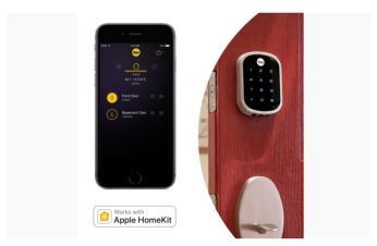
The iM1 is an add-on module for a pair of Yale products, the Assure Lock SL (YRD256) and the Assure Lock Key Free Touchscreen (YRD246). It pairs with the Yale Secure companion app to allow customers check battery status, manage up to 25 PIN codes, see current lock status, customise lock settings, name a lock or add a new lock.
