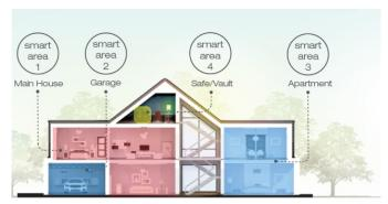
Partitioning involves the creation of zone groups in a home or building security system allowing users to arm some sections of the property while leaving other areas disarmed. The result is greater personalisation and functionality for the end user, with a one-touch solution providing access to any partition with appropriate autorisation.
