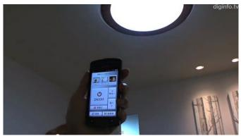
A simple LED lamp is not enough for this ceiling light fitting prototype from NEC Lighting-- it comes with integrated speaker and Bluetooth connectivity, and is controllable via Android smartphone app.
