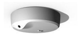
It monitors natural daylight from windows, automatically adjusting shades and lighting to reduce energy usage while maintaining the comfort and convenience. To do so it uses 2 internal photocells (one for open-loop daylight sensing, the other for closed-loop ambient light sensing) to effectively cut costs in residential, commercial or retrofit applications.
