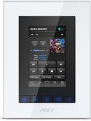
The KX3 combines an in-wall touchscreen and a control processor into a customisable and powerful easy to use unit. It is complete with proximity sensor and room status LEDs, while installation options include wired 10/100 Base-T ethernet and wireless ethernet capabilities for viewing video from network security cameras and remote programming updates.
