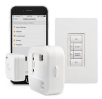
The Zūm system includes wireless dimmers, switches and sensors, all engineered to work together wirelessly. Setup requires a few taps on a keypad, dimmer or mobile app, and a single load controller supports up to 32 devices. Each device has a wireless range of 45m in every direction, and mesh networking allows communications to hop from one device to the other, with no need for interface boxes or antennae.
