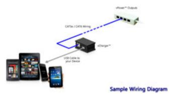
The vCharger unit draws voltage from a vPower station (via CAT5) and converts it to charge a connected USB device. Using a custom power-over-CAT5 design, it provides power for up to 100m.
