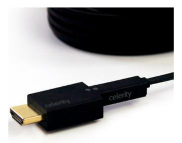
The connector at each end of the cable is fairly small (7  $\times$  25mm), allowing for easy pulling of the fibre optic pre-wire cable without need for fibre termination. One then simply affixes the detachable HDMI connector to the cable plug, making a simple 2-step process.
