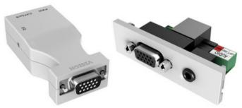
Audio passes through the transmitter, but VGA is sent to the receiver which plugs directly into the projector - via twisted pair cable up to 60 metres long. A power-over-ethernet system means only one mains power adaptor is required to power both the transmitter and receiver – and this can be used at either end.
